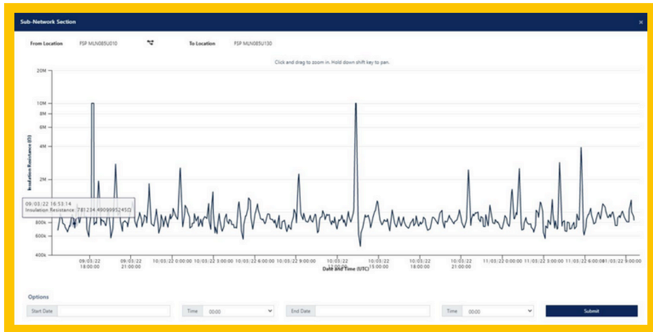
Sub-Network Section IR Measurement Captured using Temporary CableGuardian 'Roaming' Units.
